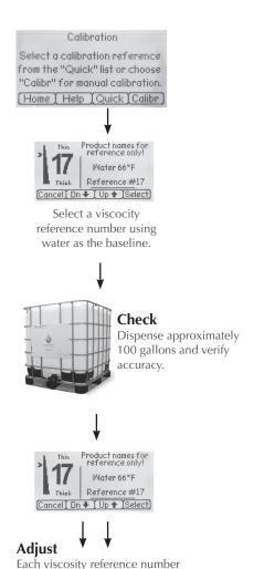
represents 1% change. (i.e.) If the meter reads high, lower the viscosity reference number. Adjust
