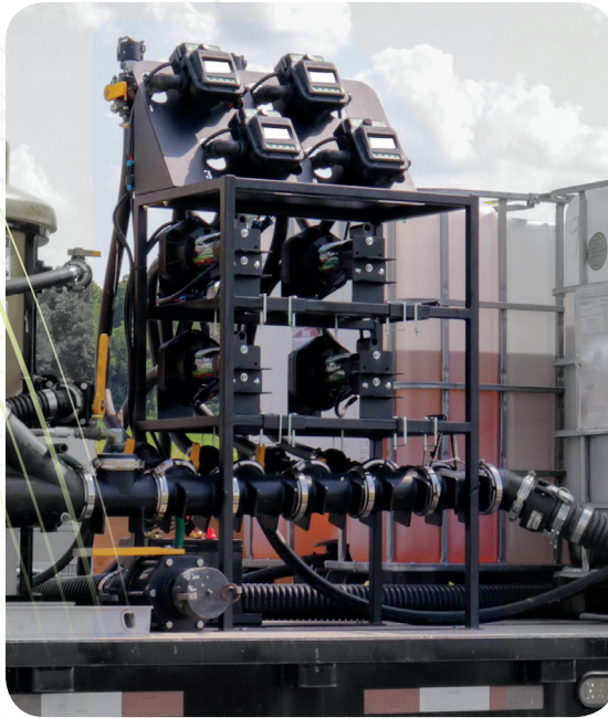
Direct inject herbicides into the carrier flow.
