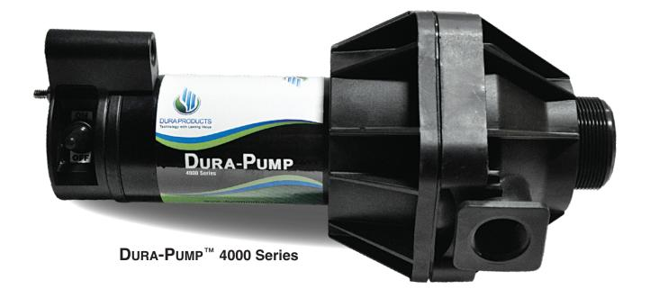
The **Dura-Pump**<sup>™</sup> **4000 Series** (DP-4000) Transfer Pump is a 12 Volt DC or 110 Volt AC, non-UL rated, self-priming, positive-displacement diaphragm pump. It is designed for non-flammable fluid transfer and recirculation. The pump includes a 20' power cord with alligator clips and an inline fuse. The pump features a 1-inch NPT inlet and a 1-inch NPT discharge port.
