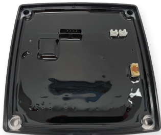
Moisture sealed circuitry.
