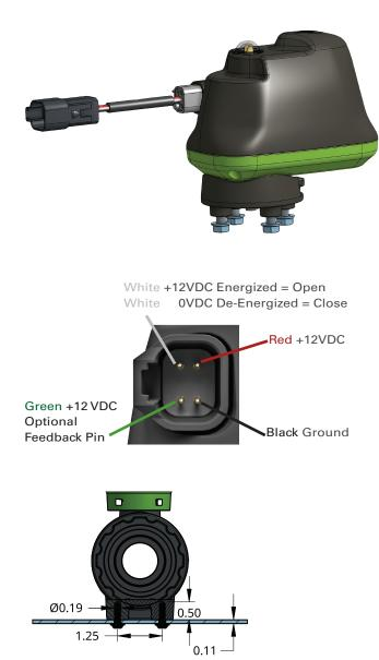
Recommended Mounting for 1" EV Hole size of 0.191" or #11 Drill Hole spacing of 1.25" Thread forming screw for plastic such as Delta PT 4.5 x 1.63 x14.5 Your mounting material +0.438" (7/16") = Recommended screw length.
