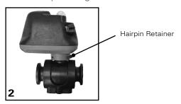
2. Remove the motorized actuator from the valve by first pulling the black hairpin retainer out of the lower neck of the actuator housing.
