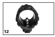
12. If the valve stem cannot be pressed back up into the bore, place the valve upside down on the work surface, with the valve resting on the actuator mounting head. A non-marring tool handle of plastic or wood can be placed through the valve body. This will allow additional force to be applied evenly on both sides of the valve to aid full insertion of the stem.
