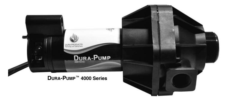
The **Dura-Pump**<sup>™</sup> **4000 Series** (DP-4000) Transfer Pump is available as a 12 Volt DC or 110 Volt AC, non-UL rated, self-priming, positive-displacement diaphragm pump. It is designed for non-flammable fluid transfer and recirculation. The 12 Volt DC pump includes a 20' power cord with alligator clips. The 110 Volt AC pump includes a 6' 6" power cord with 3-prong plug. Both pumps include an inline fuse and feature a 1-inch NPT inlet and a 1-inch NPT discharge port.
